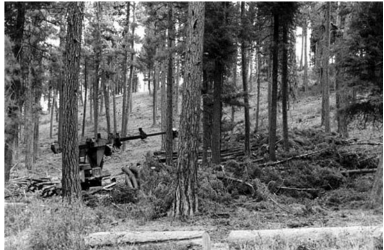
A feller-buncher on a restoration project on the outskirts of Missoula removes all stems in one pass, eliminating the need for pre-harvest hand slashing. The prescription – to leave 10' between the crowns of the biggest trees – will reduce hazardous fuels. Harvested trees are sold as sawlogs, pulp logs and hog fuel. The Trench Society hopes to use this harvesting method on the Waldo North project.
